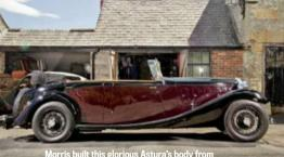
scratch using a home-made wheeling machine
